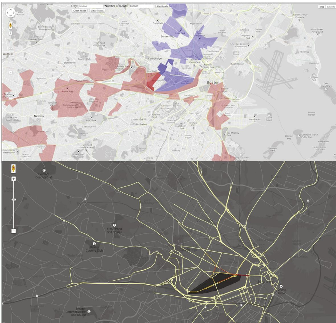
**Fig. 8.** Two screen images from the visualization platform. (a) The trip producing (red) and trip attracting (blue) census tracts using Cambridge St., crossing the Charles River in Boston. (b) Roads used by trips generated at the census tract including MIT. (For interpretation of the references to colour in this figure legend, the reader is referred to the web version of this article.)
