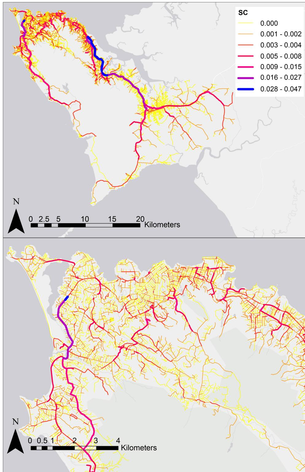
FIGURE 3.3: Service Centrality for all facilities shows a distribution throughout the network that is not strongly directional. The complex interaction of shortest paths to multiple facilities often highlights road segments as important which may not appear so otherwise
