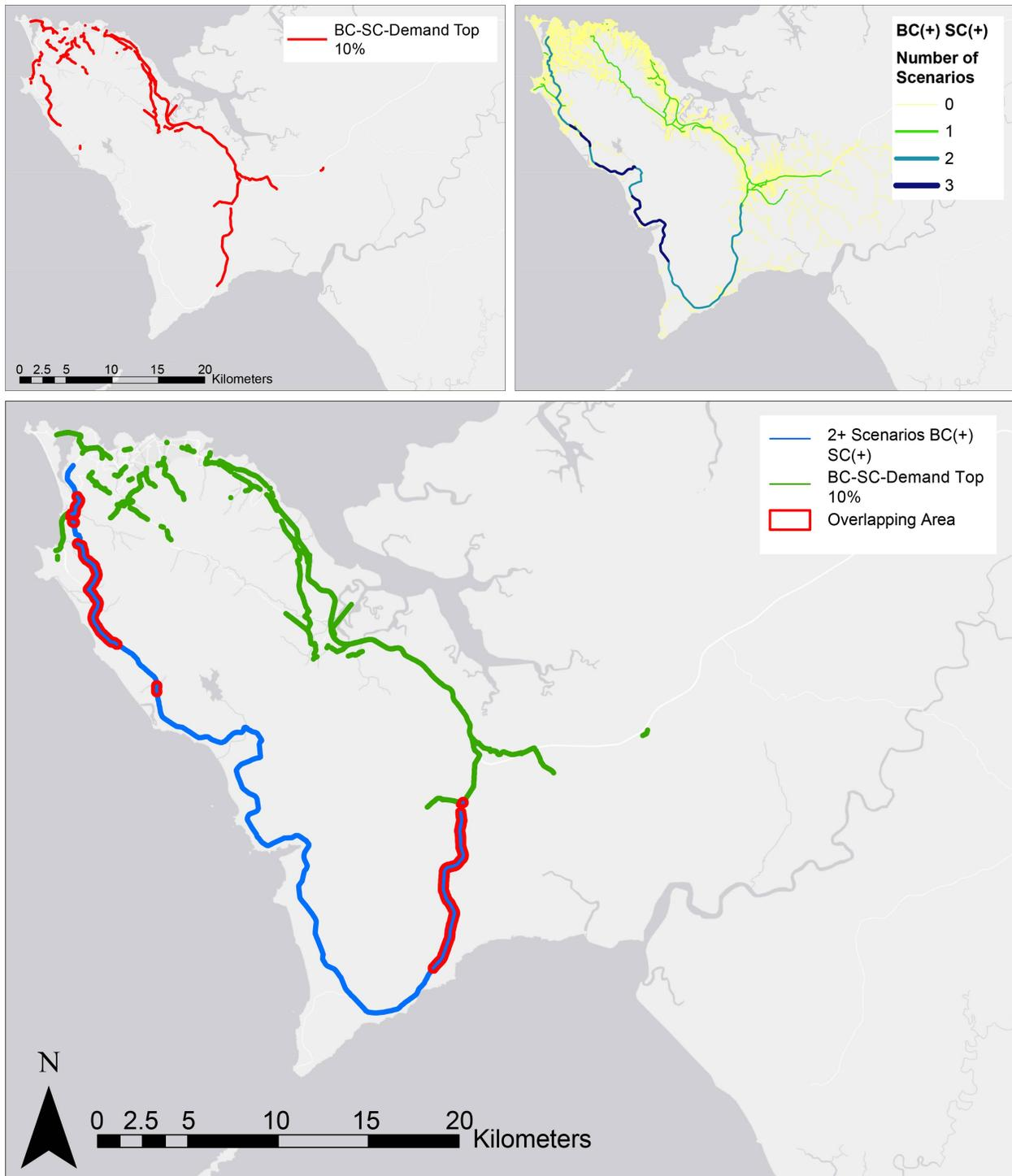
FIGURE 4.5: Selection process for critical road network areas: a) road network facilities in the top 10% percentile of both Demand Weight and SC (corresponding with Figure A.17 Critical category, red); b) road network facilities characterized by the number of Major Flooding Hazard scenarios which resulted in increases to BC and SC (corresponding with Figure 4.3 Demand(+) SC(+) category, blue); c) road network facilities which are indicated in both a) and the higher values (2 and 3) of b
