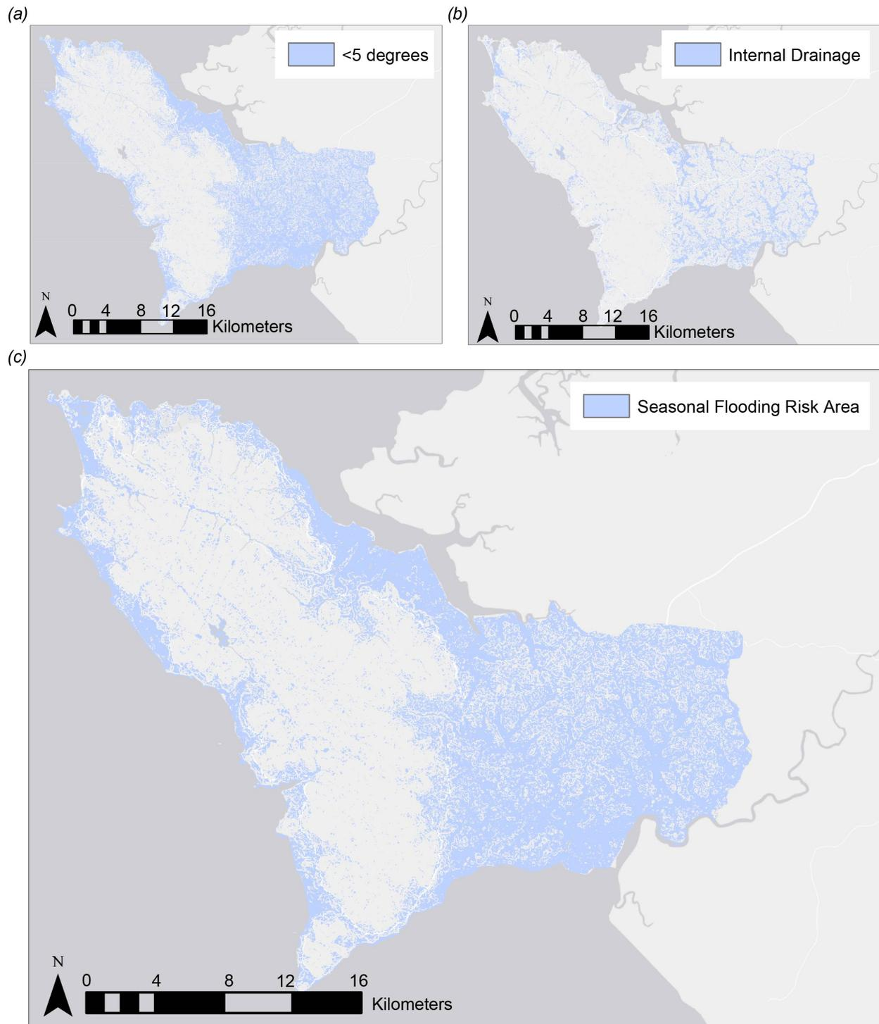
FIGURE A.21: Seasonal Flooding Hazard Extent, a) Areas with slope of less than five degrees; b) Sinks, or areas with no outlet for drainage, c) Union of 11a) and 11b), representing the extent of expected seasonal flooding risk
