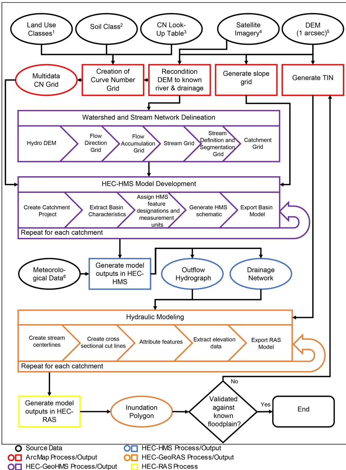
FIGURE 3.4: Method to estimate the extent of Major Flooding Hazards
