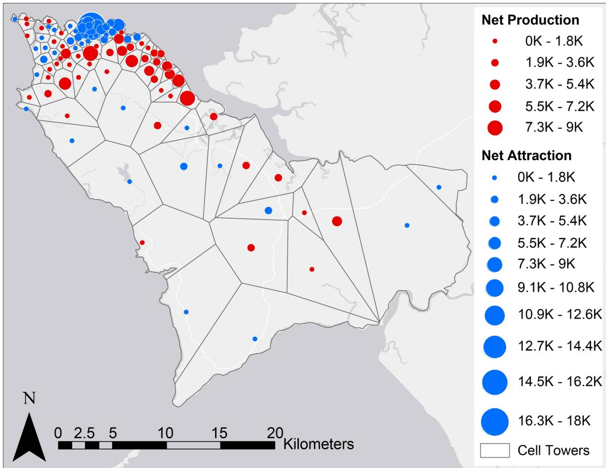
FIGURE A.18: Net trip production and attraction set within a Voronoi diagram based on cell tower location shows likely job attraction areas (North, blue dots) and residential production areas (Northeast coast, red dots)
